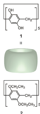
Figure 1. Chemical structures of (a) per -hydroxylated (1) and per -ethylated (2) pillar[5]arenes and (b) viologen-based axes containing an adamantane and azobenzene moiety at either end (3), dodecyl chains (4), or adamantane moieties (5) at both ends.
